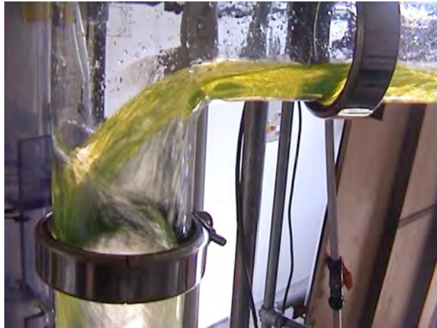
Figure 1 Water discharging from a branch Heriot-Watt University
