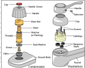
sary). Using a little petroleum jelly may also make screwing the stem back in place a little easier.
