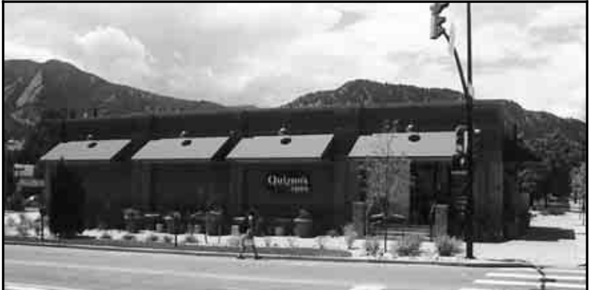
Where a parking facility shares a site with a building, place the parking facility at the rear of the site or beside the building. This store and gas station located on a corner lot has kept the auto-oriented portion of the use to the rear of the site, thereby preserving the building edge at the sidewalk.
