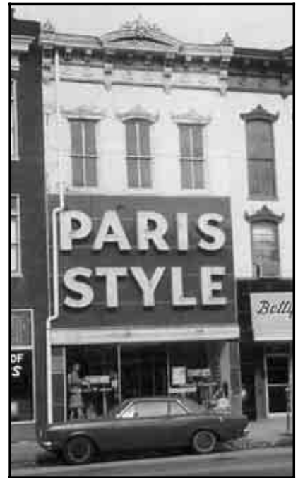
Any sign that visually overpowers the building or obscures significant architectural features is inappropriate.
