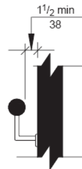
Fig. 505.5 Handrail Clearance
